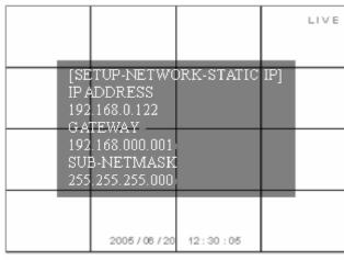
Fig3.2.28 Setup static IP
